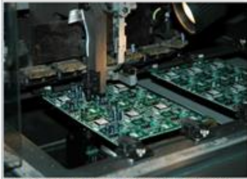
Full automation insertion machine (AI/RI)
