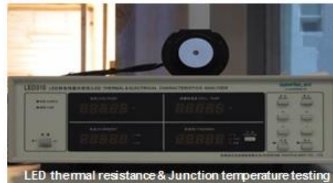
LED thermal resistance & junction temperature testing
