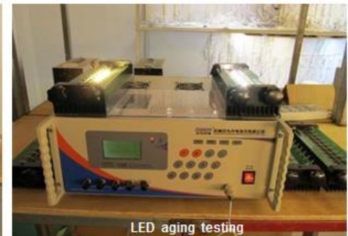
LED aging testing
