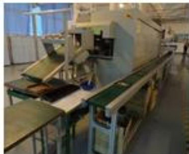
Wave solder carrier return automation
