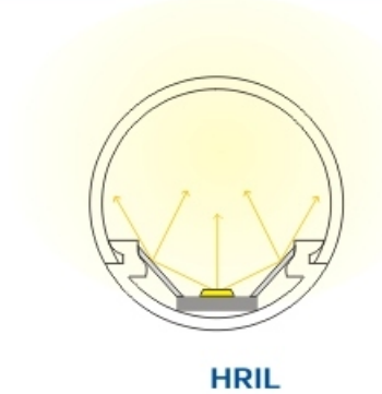
Glaring LED light reflected by the MCPET before reaching the eyes of end users
